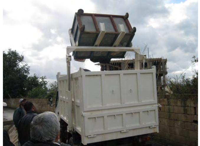
New garbage truck in action. Project funds also covered the cost of new disposal bins and the repair of existing bins (fitting with new wheels, metal sleeves for hydraulic arms on truck, etc.)
